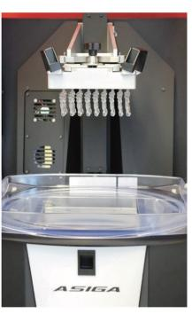
▲ ABUVE: Dental splints printed on an Asiga PRO2 3D printer using FreePRINT Splint material supplied by DETAX. Picture courtesy of DETAX GmbH.
